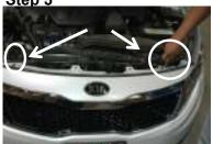
Remove (2) 10mm bolts located on each side of the bumber
