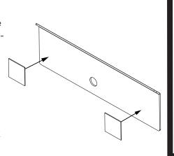
Apply single sided adhesive pads to this side of spacer.
