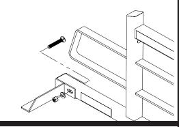
Fasten RealTruck Backrack Assembly to the Stake pocket bolt as shown.
