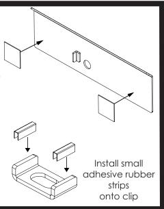
Apply single sided adhesive pads to this side of spacer.
