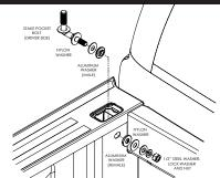
Fasten RealTruck Backrack to the rail mount bracket. Finger tighten at this stage.
