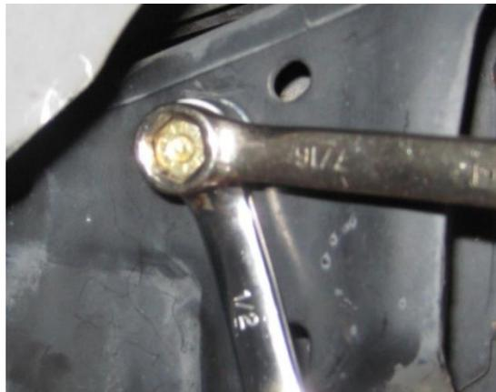
Y. Remove the screw, washer, and flange nut. The Threaded Insert should now be rigidly fixed in the hole as shown below.
