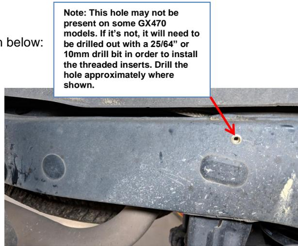
Note: This hole may not be present on some GX470 models. If it's not, it will need to be drilled out with a 25/64" or 10mm drill bit in order to install the threaded inserts. Drill the hole approximately where shown.
