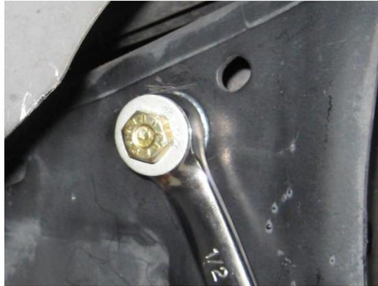
X. While keeping the Threaded Insert flange firm and parallel against the frame rail, tighten the screw using a 7/16" box end wrench or socket. Turn it 2.5 rotations to set the Threaded Insert. Tightening in 1/4 turn increments tends to work well.
