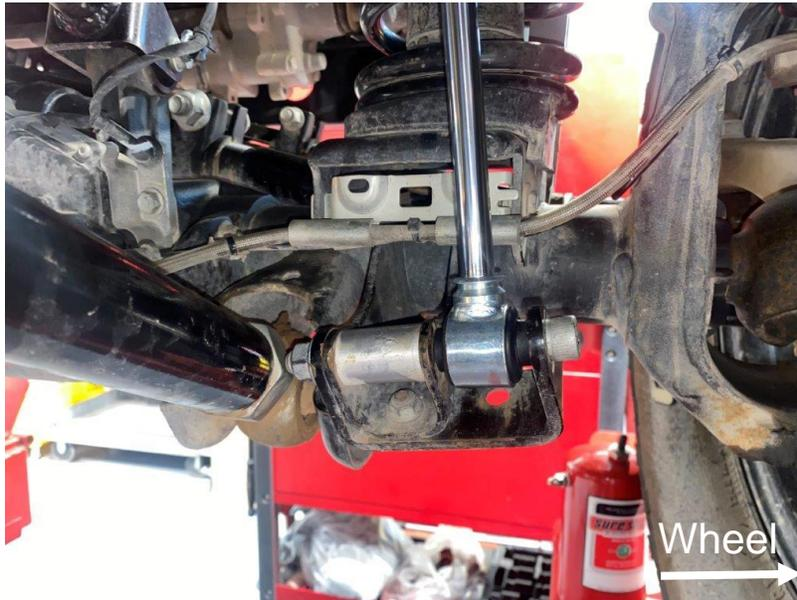
**Figure 14: Passenger Side Bottom Mount**
