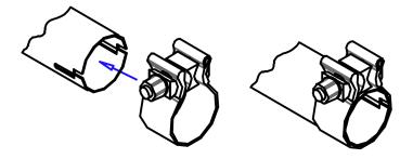
WARNING: Use extreme caution during installation. Torque all fasteners according to manufacturer's torque values and tightening sequence. <u>DO NOT</u> use air impact tools to tighten fasteners on Borla Performance Exhaust Systems. Use of such tools may result in bent flanges or gasket contact areas leading to exhaust leaks.
