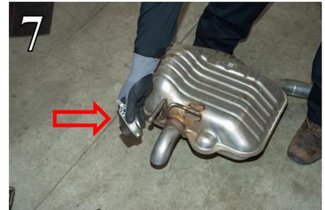
7. With the original exhaust on the shop floor, remove the rear muffler hanger brackets. **Note which side each bracket belongs to, as they will be installed the on the opposite side in order to mount your Borla Performance exhaust system (figs. 6, 7).**
