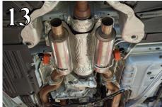
WARNING: Use extreme caution during installation. Torque all fasteners according to manufacturer's torque values and tightening sequence. <u>DO NOT</u> use air impact tools to tighten fasteners on Borla Performance Exhaust Systems. Use of such tools may result in bent flanges or gasket contact areas leading to exhaust leaks.
