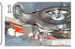
Note: With a used vehicle, we suggest a penetrating spray lubricant to be applied liberally to all exhaust fasteners and allowing a significant period of time for the chemical to lubricate the threads before attempting to disassemble.
