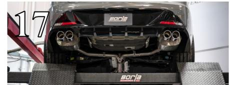
**WARNING:** Use extreme caution during installation. Torque all fasteners according to manufacturer's torque values and tightening sequence. **DO NOT** use air impact tools to tighten fasteners on Borla Performance Exhaust Systems. Use of such tools may result in bent flanges or gasket contact areas leading to exhaust leaks.
