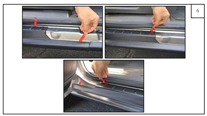
Set part in place on vehicle. Remove all red tape liners. Do not forget tape liners on bottom of part. Apply **FIRM** pressure to mounting locations to affix to truck.
