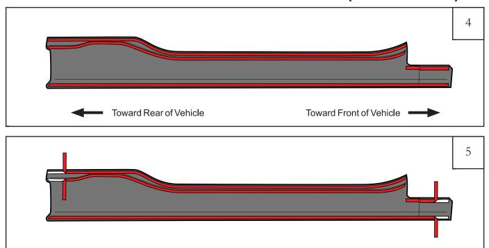
Peel back roughly 3" of red tape liner from the pieces of tape on the back side of rear part. Make sure red tape liner will be accessible when part is attached to truck.
