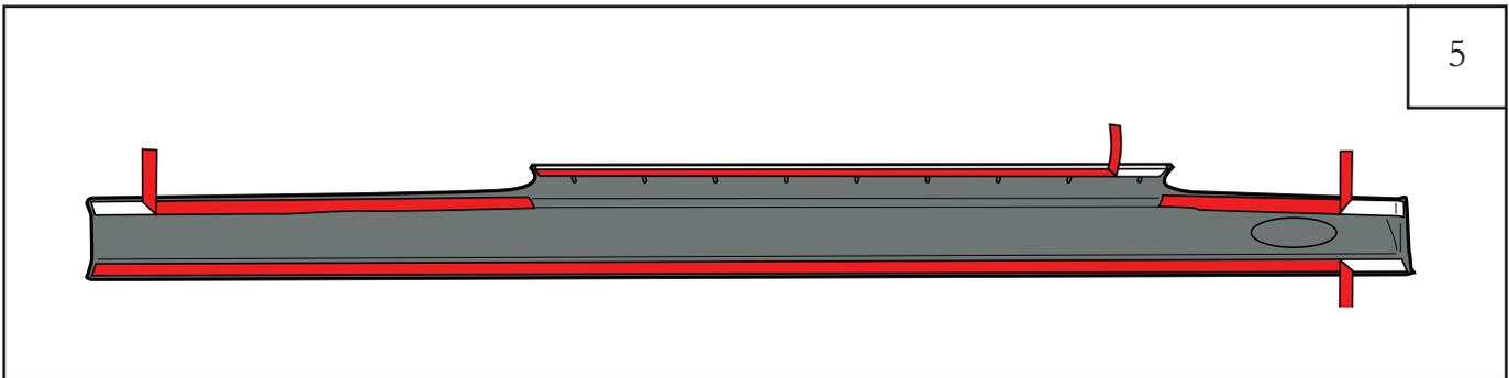
Peel back roughly 3" of red tape liner from the pieces of tape on the back side of rear part. Make sure red tape liner will be accessible when part is attached to truck. Tape layout may be different on Crew Cab part.
