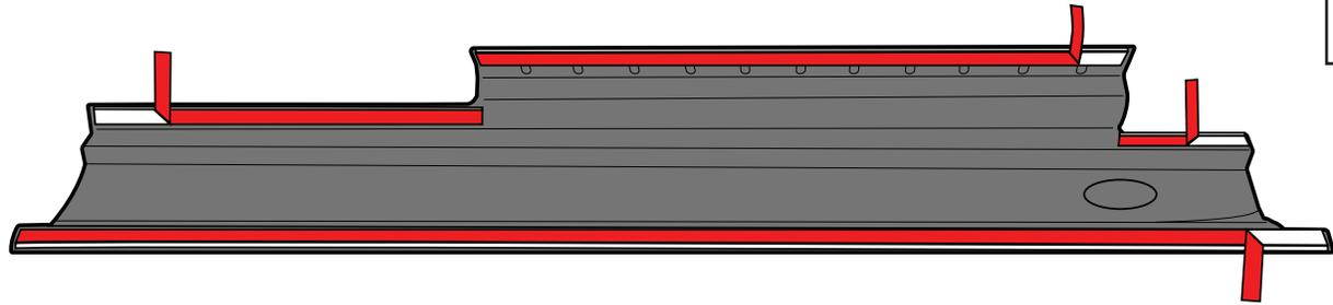
Peel back roughly 3" of red tape liner from the pieces of tape on the back side of rear part. Make sure red tape liner will be accessible when part is attached to truck.
