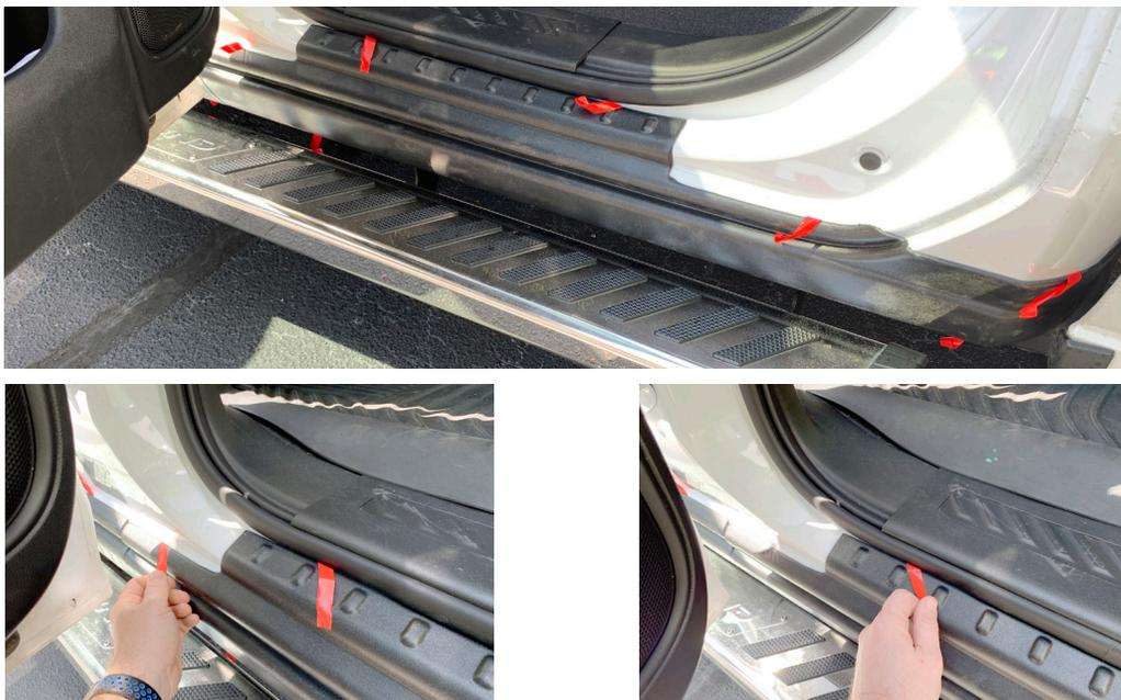
Set part in place on vehicle. Remove all red tape liners. Apply **FIRM** pressure to mounting locations to affix to truck.
